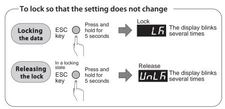
You can lock or release only when the display shows the rotation speed.
