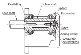
• When the load shaft is not stepped
