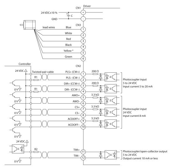
\* No lead wire is provided for motors of Model A. Do not connect anything to the pin number 5.
