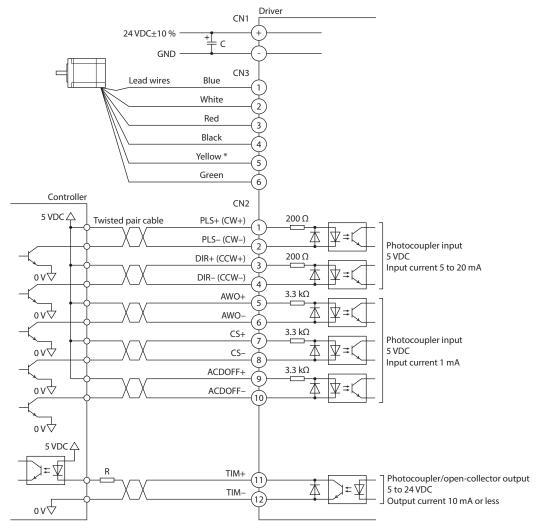
$^{\ast}$  No lead wire is provided for motors of Model A. Do not connect anything to the pin number 5.
