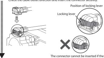
The connector cannot be inserted if th locking lever is turned down.
