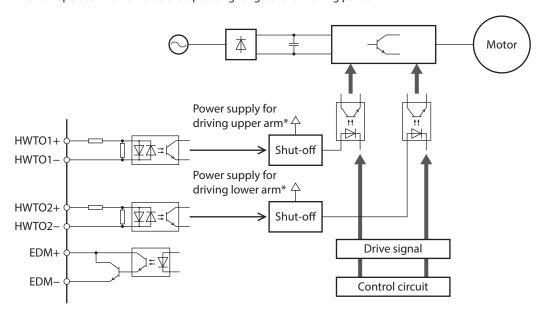
\* Turning the HWTO1 input OFF causes the upper arm drive signal of the inverter circuit to shut off. Turning the HWTO2 input OFF causes the lower arm drive signal of the inverter circuit to shut off.
