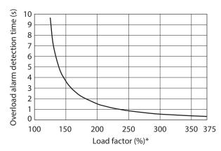
\* This indicates the motor output power presently generated as a percentage of the maximum output power in the continuous duty region.
