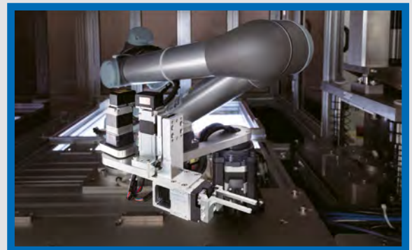
„Custom-Built” SCARA robot that uses the limited space under the arm of the industrial robot
