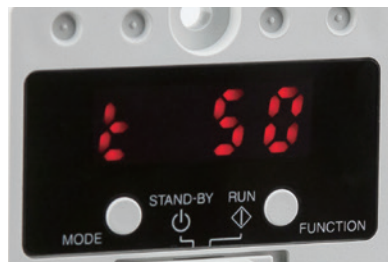
Indication at a load factor of 50%
